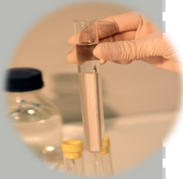
Insertion of sample in the contaminant solution
